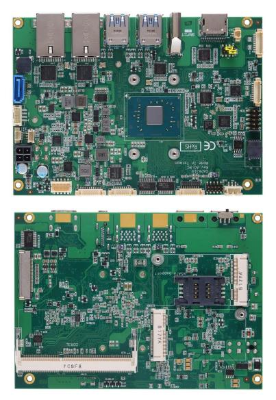
The CAPA315, a 3.5" board, supports Intel<sup>®</sup> Pentium<sup>®</sup> N4200 and Celeron<sup>®</sup> N3350. It delivers outstanding system performance through high-bandwidth interfaces, multiple I/O functions for interactive applications and various embedded computing solutions.
