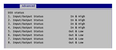
Once it is enabled, you can load manufacture default and access to the DIO status sub screen to set output or input, see image below.
