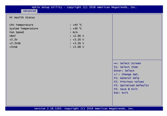
This screen displays the temperature of system and CPU, fan speed in RPM and system voltages (VBAT, +3.3V, +3.3VSB and +5VSB).
