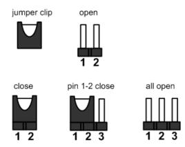
Properly configure jumper and switch settings on the CAPA312 to meet your application purpose. Below you can find a summary table of jumpers, switch and onboard default settings.
