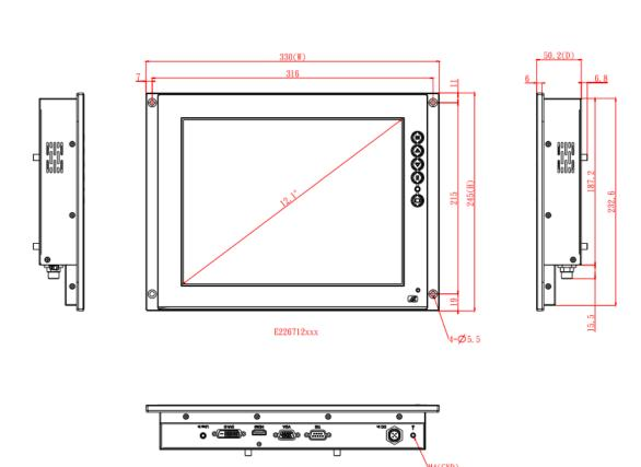
The following diagram show the VESA mounting and cut-out dimension of P712
