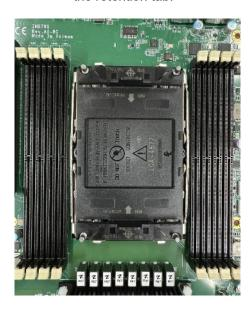
**Step 2** Insert the CPU onto the CPU clip and align upper left pin mark on the CPU clip.
