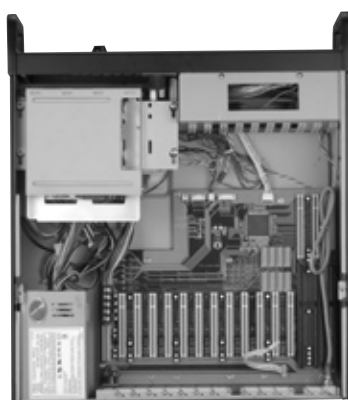
Top view with 14-slot backplane
