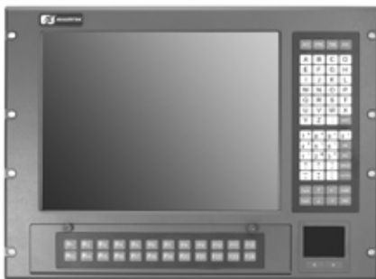
Built-in 24 function keys and 66 membrane keypads
