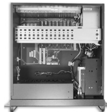
Top view with 14-slot backplane
