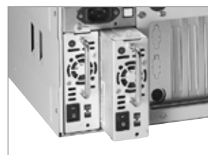
Optional hot-swap redundant power supply
